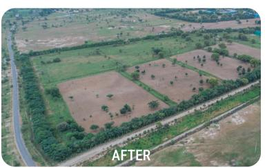
**RECHARGING AQUIFER -** Water that percolates through lakes, swales, and chaukas gets **naturally filtered** through the ground and **replenishes the aquifer,** increasing the water table and making the water suitable for consumption. There are over **50 wells** in and around Dhun that have started receiving water again after being dry for the past 10 years. The **TDS levels have decreased by 26 times.**
